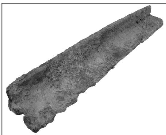
Fig.2. Plate rail from another early Outram line at Codnor Park, kindly donated to the Butterley Gangroad Project by the Portland Path Project. The rail weighs 38lb (17.2kg).
